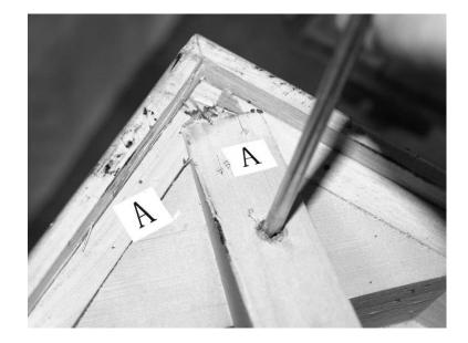
3. Fix the top of the oblique beam to the upright post by screwdriver. Pay attention to the mark in the top of the oblique beam, make sure the mark is corresponding to the upright post. See figure below:
