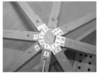
4. Repeat the step 2~3 and tight the other oblique beams to the correct position. See figure below:
